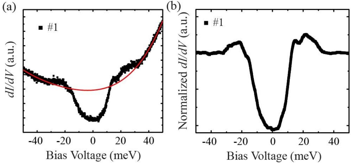
Figure S1| (a) Original  $dI/dV$  spectrum of 1uc-FeSe/STO at point #1 marked in Fig. 3. The background for normalization is fitted by a polynomial function and plotted in the red line. (b) Normalized  $dI/dV$  spectra at point #1 as shown in Fig. 3(c). The original  $dI/dV$  spectra are normalized by the red line in (a) and smoothed by the average of adjacent 20 points.
